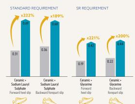
Slip resistance test according to EN ISO 20344:2021,
